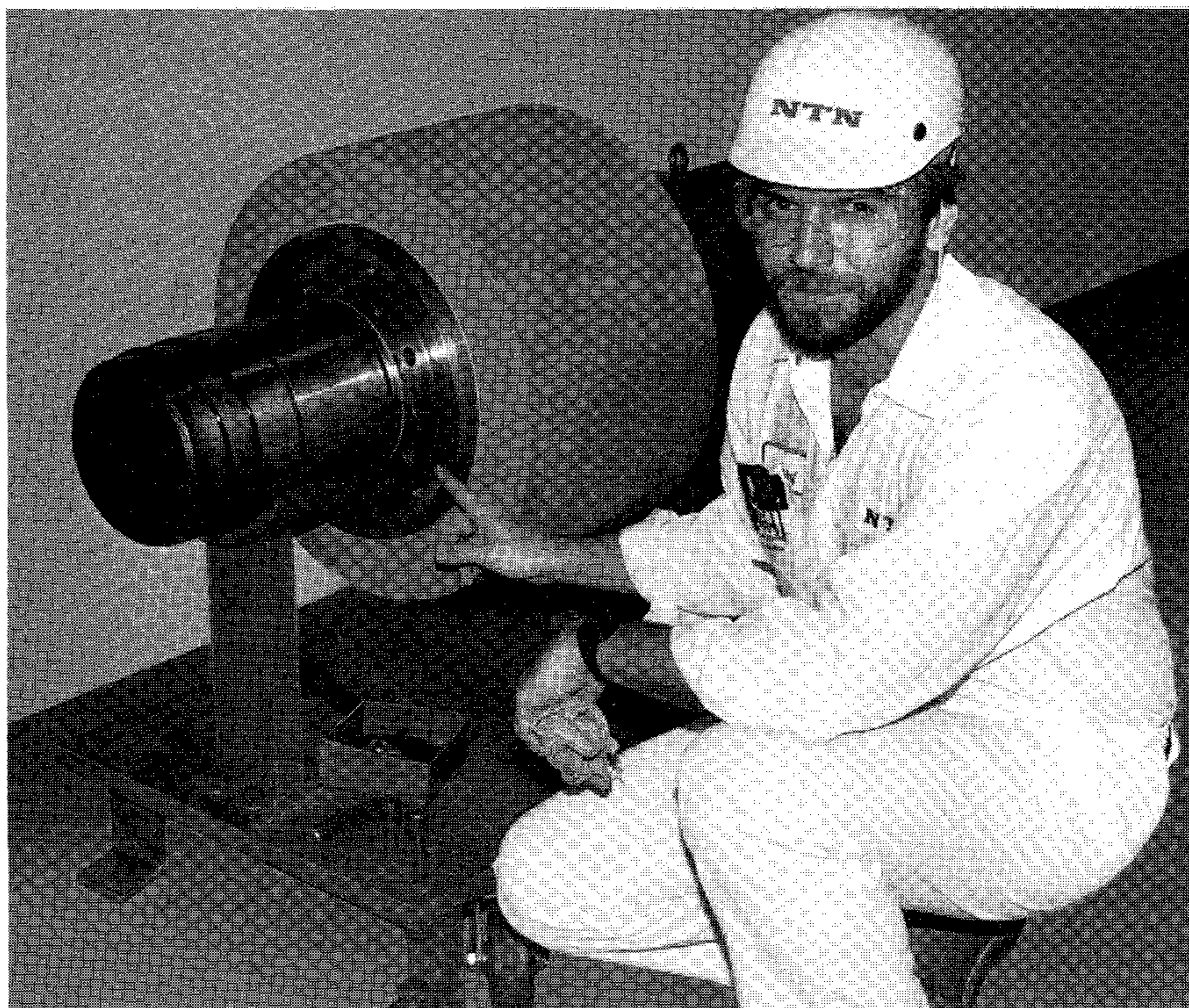
Bearing quality greatly depends upon the quality of the grinding wheel. By permanently monitoring vibrations from the grinding wheel, a tight check can be kept on its condition
